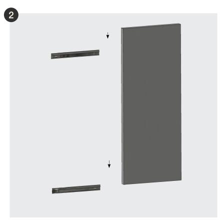
The DAMPA® Silent Board panels are installed by lowering the upper edge of the panel, along with the crossing rail on the back, onto the wall carriers.
