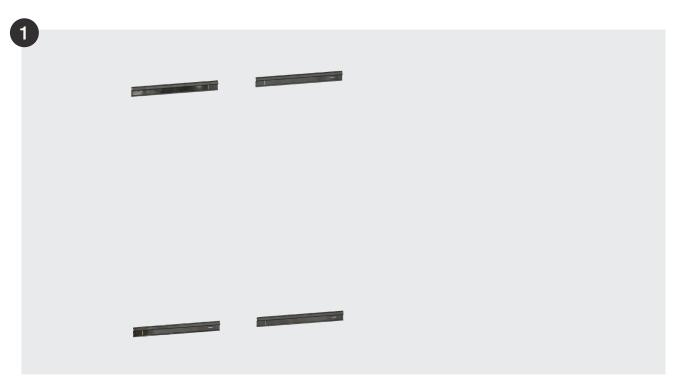
The top wall carrier is initially installed by positioning it so that its upper edge aligns with the desired height of the wall panel. The wall carrier is mounted level on the wall using flat-head screws.
