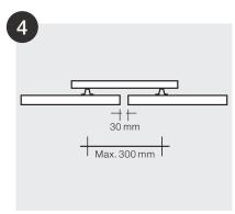
When installing ceilings requiring panel lengths greater than 6 m, jointing can be achieved by forming a desired gap between the ends of the panels.
