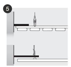
To prevent movement of the ceiling, modular carriers are braced against the wall. The first and last modular carriers should be braced at right angles approx. every 2000 mm.
