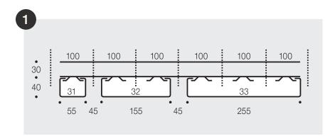
Installed in the same modular carrier all types have an open gap of 45 mm.
