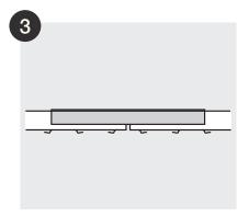
The modular carriers are joined using Carrier Splice No. 26.
