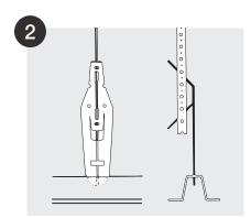
Adjustment Clip No. 5 with Hanger No. 5 is located into the slots provided in the modular carrier.
