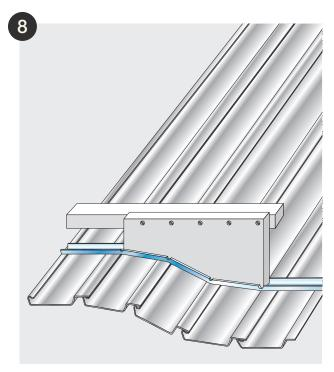
Concave or convex curved surfaces to a minimum radius of 500 mm can be achieved using Modular Carrier No. 44.
