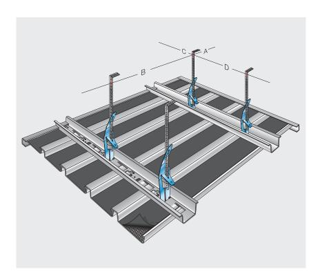
After fixing of the perimeter trims, the modular carriers are suspended.
