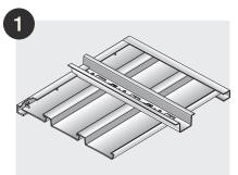
Edge Trim Type 1 is used at right angles to the ceiling units and Edge Trim Type 2 parallel to support cut units.
