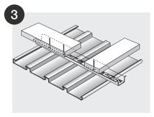
To prevent movement of the ceiling, modular carriers are braced against the wall with timber battens as shown.
