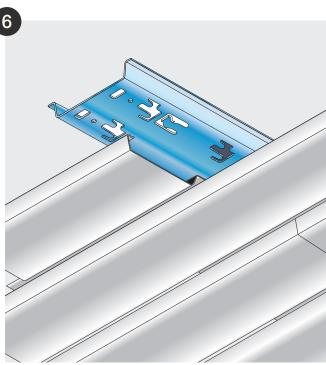
Closed joints are formed under Modular Carrier No. 43 (double carrier). Hangers must be fastened alternatively to both sides of the carrier to prevent twisting.
