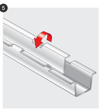
Modular Carrier No. 40 is provided with pre-punched lugs and cut-outs for modular splicing.
