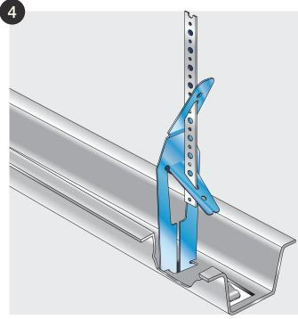
Adjustment Clip No. 5 is located into the slots provided in the modular carrier. Minimum suspension height is 170 mm.
