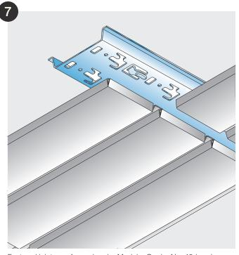
Featured joints are formed under Modular Carrier No. 43 (can be supplied painted). The maximum width of the open joint is 50 mm.
