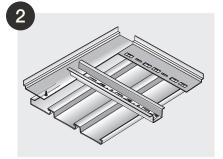
Angle Runner No. 1 with clips is used at right angles to the units (maximum distance to the first modular carrier 1600 mm) and Angle Runner No. 2 is used parallel to the units.
